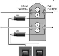
error while accelerating or decelerating, thereby eliminating web droop between the slitter/scorer and infeed pull roll sections.
