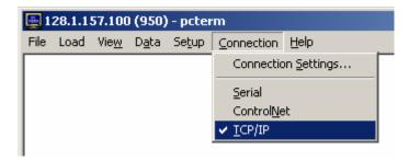
The **Connection** menu item lists the available types of communication PCTerm supports. This version currently supports standard serial communication, ControlNet™ talk-through to UNICO controllers, as well as TCP/IP socket connections. The currently selected connection type is displayed with a check and is changed by clicking on an unchecked selection. Multiple instances of PCTerm may be opened and configured for different connections.
