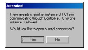
Clicking **Yes** will open a new instance of PCTerm configured for serial communication, while clicking **NO** causes the following dialog to appear.
