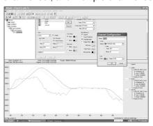
channel set can be sampled at different sample rates. Sampling can be continuous or triggered by complex user-defined trigger conditions. Captured data can be read and displayed by an HMI in real time, subject to limits of the serial connection, or buffered in the drive for subsequent retrieval and analysis. An optional memory expansion module is also available that allows multiple sample sets to be stored on a removable SD memory card.
